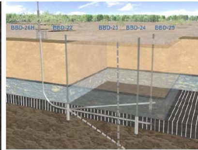
Figure 5a: Bi-lateral wells, with shield wells Figure 5b: Tri-lateral well cross section Source: Eastern Star Gas Limited
